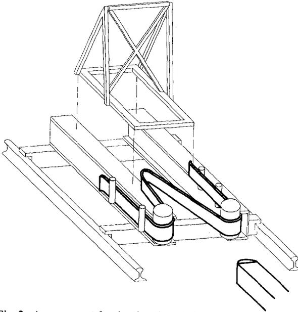
Fig. 2. Arrangement for deceleration of the sled
