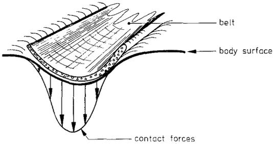
**Fig. 7.** Effective contact area between belt and body
